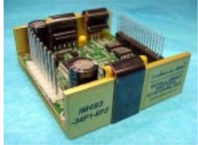
This option may be solder-mounted or the pins may be wire-wrapped for interfacing.
