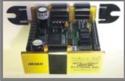
Figure D.2-A: Clips being installed on an IM4831
